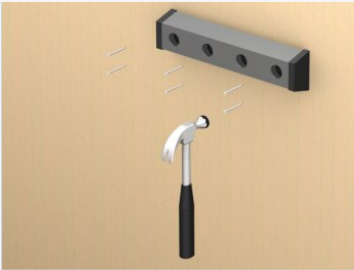
3. Trapezoidal batten with reinforcement bars installed
