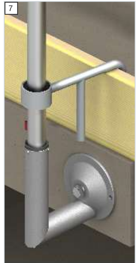
Screw-in side grip + kerb plank grip
